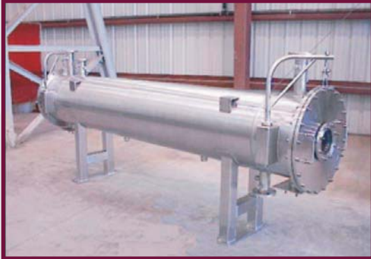
Heat Exchanger with stainless tubes and shell with a #4 exterior polish.
