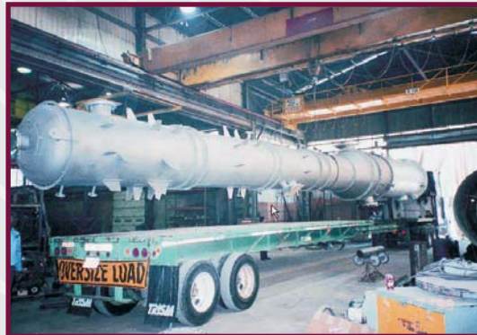
Alloy 2205 Trayed Column 48" to 72" variable I.D. by 49' OAH.
