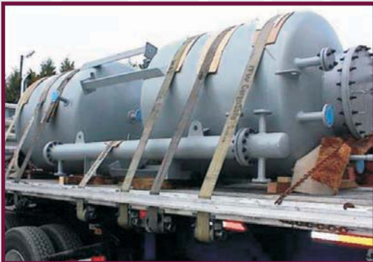
Alloy Vessels and heat exchanger painted due to corrosive plant environment.
