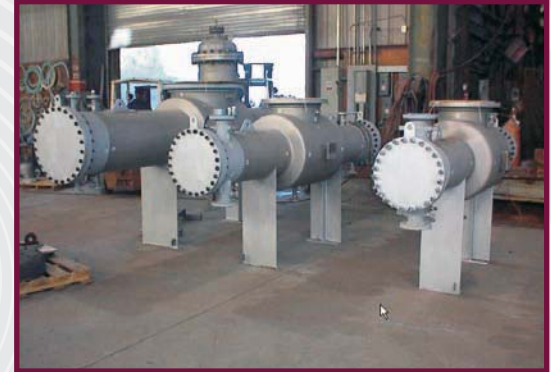
Heat Exchangers with Hastelloy C-276 tubes and shell.
