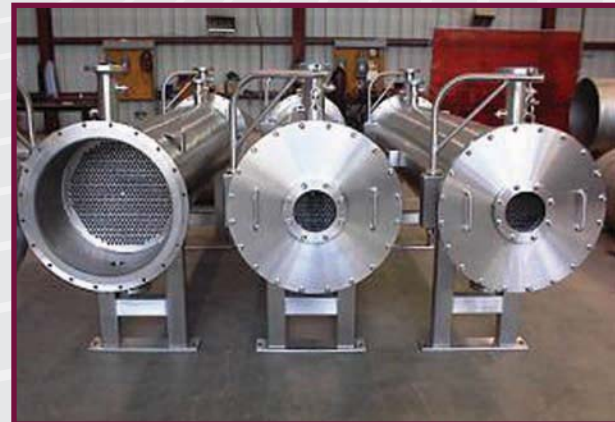
(Below) Stainless Steel Heat Exchangers.
