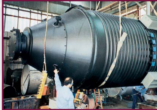
Reactor Stainless with double internal pipe coils, half pipe jacket on shell, conventional stainless jacket on cone, 100% x-ray for lethal service.
